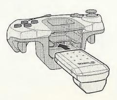
When the Jump Pack/Vibration Pack is inserted into Expansion Socket 1 of the Sega Dreamcast Controller, the Jump Pack/Vibration Pack does not lock into place and may fall out during game play or otherwise inhibit game operation.
